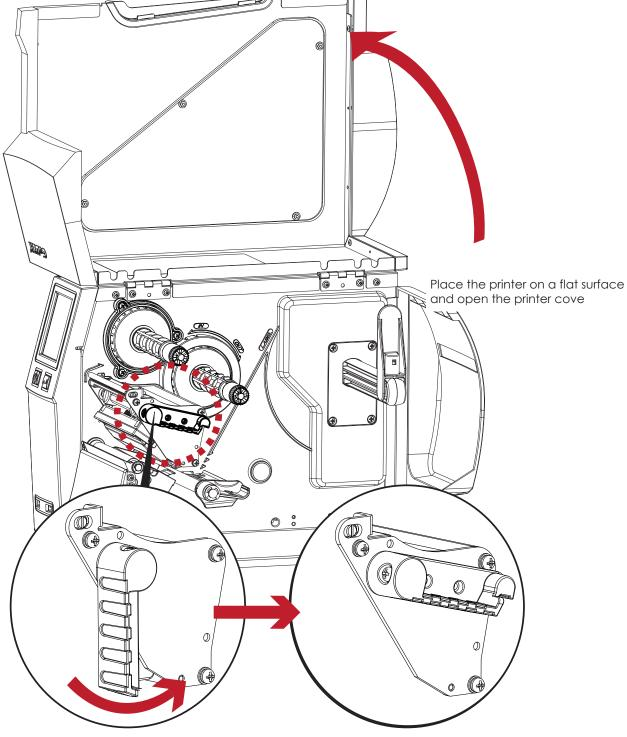
Turn it anticlockwise to a top right position as shown in the illustration
