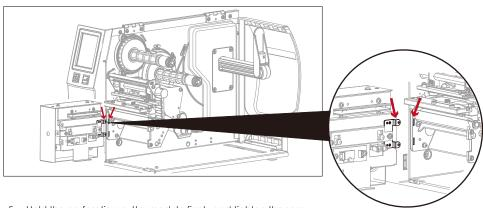
5. Hold the perforation cutter module firmly and tighten the screw
