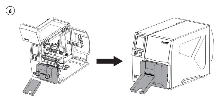
1. Snap the ticket tray to the cover of cutter to complete the installation.
