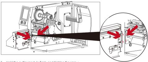
5. Hold the cutter module firmly and tighten the screw
