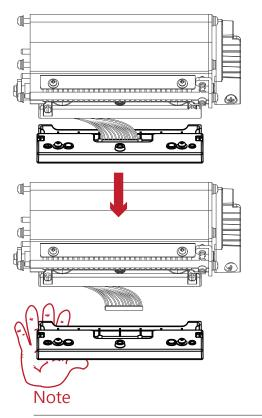
Hold the print head module , pull out the TPH cable smoothly. To install TPH module, follow the reverse order.
