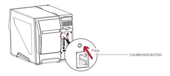
Press C-button for 2 seconds, it will make an auto-sensing to calibrate the label and ribbon's parameters.
