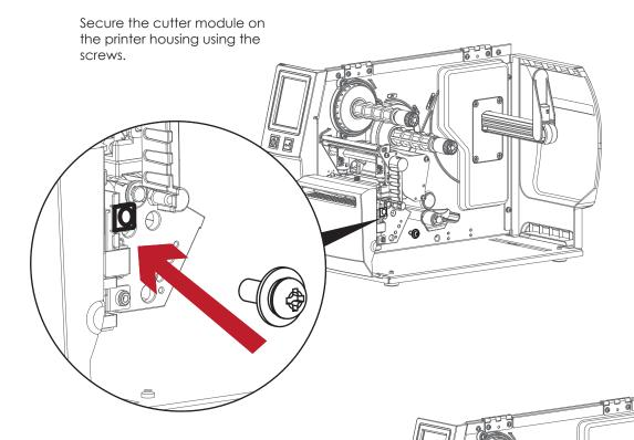
Finish the cutter module installed.
