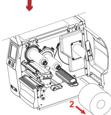
Step 2. Pull the Liner roll out
