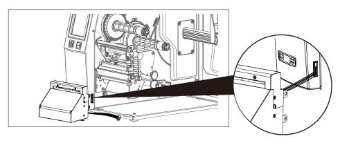
4. Insert the cutter module to dock with the printer
