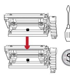
using a screwdriver or a coin to loosen the screw
