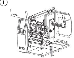
1. Assemble the Platen module bracket.
