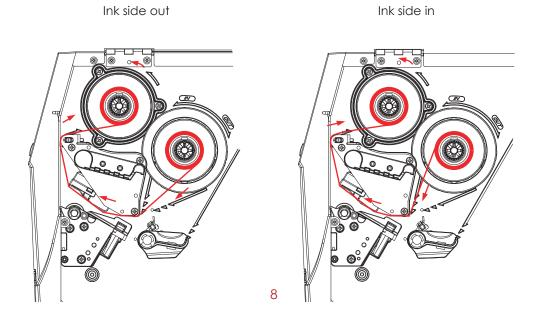
Pass the ribbon under the print head and back up on the other side. Attach it to the empty ribbon core.
