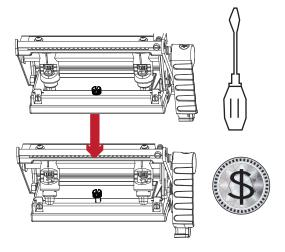
using a screwdriver or a coin, loosen the screw to take out the TPH module.
