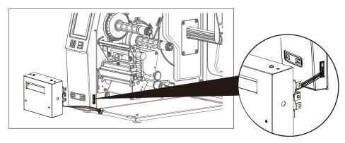
4. Insert the perforation cutter module to dock with the printer
