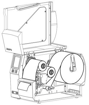
Now load the label roll into the printer and close the printer cover.
