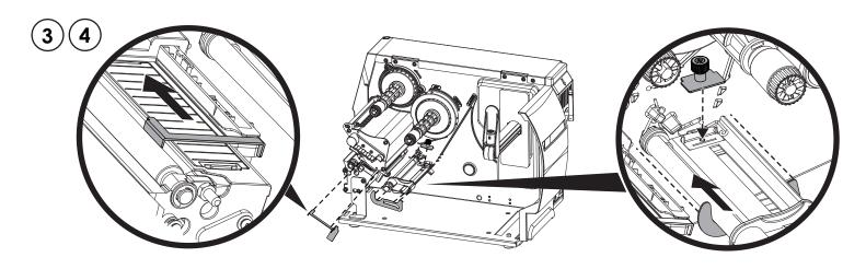
1. Install the label bracket and the label holders respectively. During the installation, push the parts to the left end and fix them with double-sided tape.
